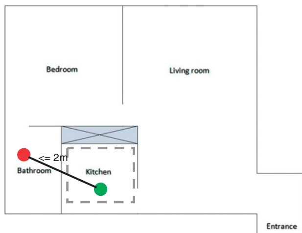
Figure 5. Small room problem. The kitchen is very close to the bathroom so the tag was identified as in the bathroom (green circle marked the current location and the red circle represents the location calculated by the server).
