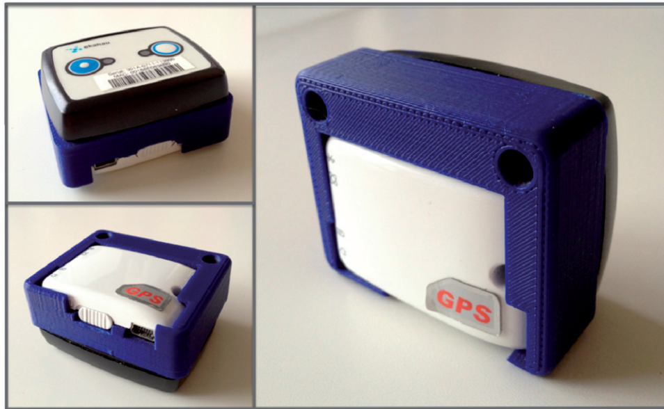
Figure 1. The sensing tag with dimension of 54 mm × 45 mm × 26 mm. Left-top : GPS logger for the outdoor tracking. Left-bottom : WiFi tag for the indoor tracking. Right : different view of the tag.
