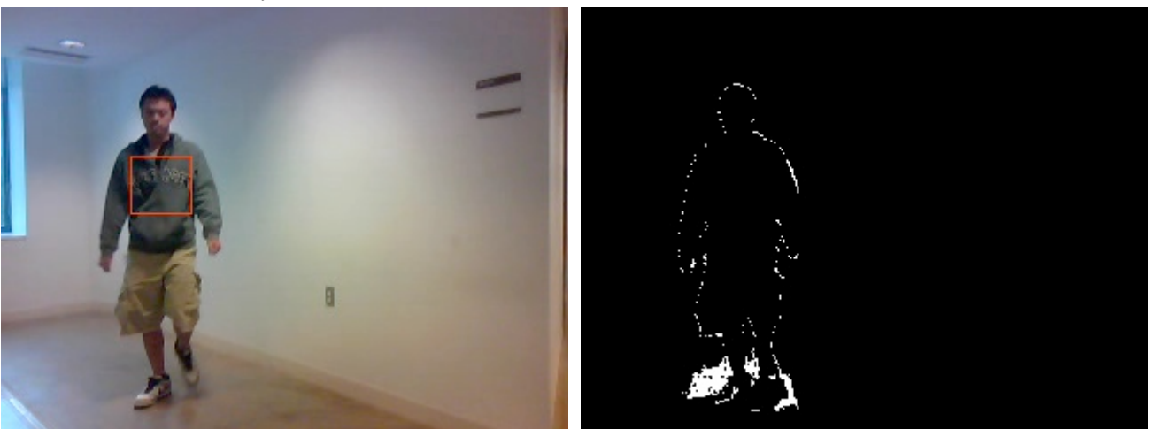
Fig 4. Original image (left) and the shadow detection (right)
